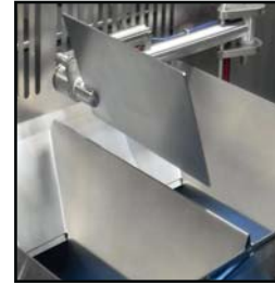
Hopper Feed Diverter
