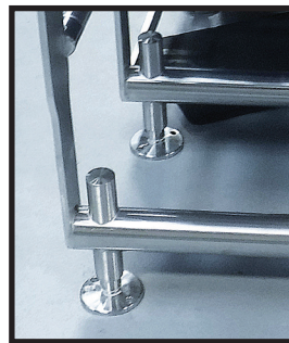
Adjustable Feet With No Exposed Threads
