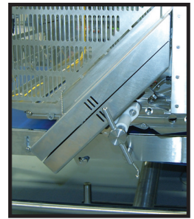
Easy Blade Tensioner With Indicator
